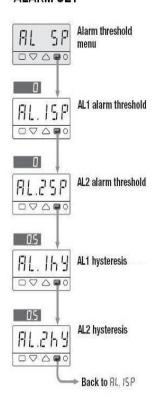
: Setting of alarm setpoint for alarm 1, e.g. 200 (°C)
