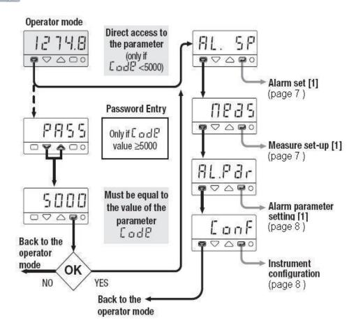
To access all levels, a password has to be entered after pushing than 5000). This is done by holding down the buttons and the instrument automatically selects ones, tens, hundreds and thousands and selectably increases or decreases.
